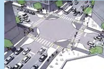
Figure 4-7: Protected intersection concept
