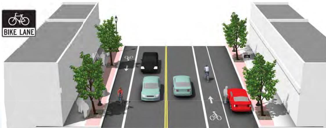
Figure 2-10: Typical bike lane cross section with and without parking
