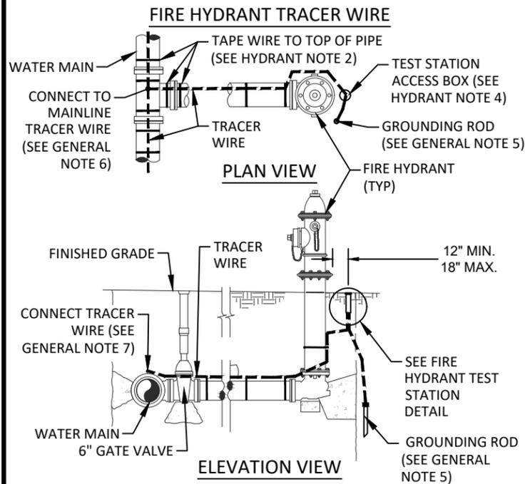
**FIRE HYDRANT & STANDARD MFR TEST STATION DETAIL**
